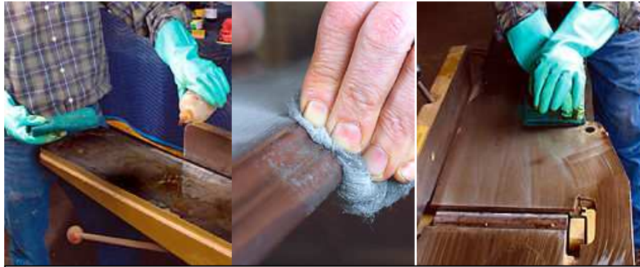
To remove rust from a tool bed, apply paste wax, splash on some mineral spirits (left) and then rub away with abrasive pads in successive grits (right).
